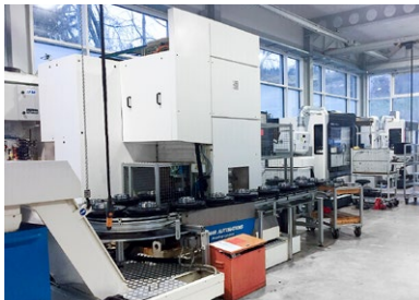
Pallet pool for unmanned production
