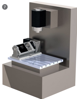
7 4 th + 5 th axis, 2-spindle, Y-mounting (crosswise)
