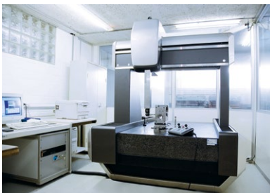
Measuring a housing on a 3D measuring unit
