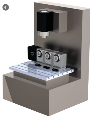
4 4 th axis, 3-spindle, X-mounting (lengthwise)
