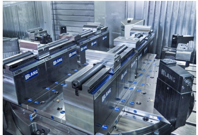
Machine-tools: DMG Mori DMF 360, customised Makro-Grip® Ultra solution with a clamping range up to 1.000 mm
