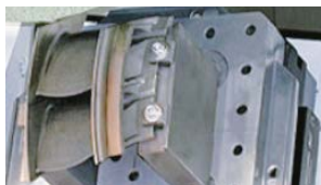
Turbine blade on GPS 240 – Source: System 3R
